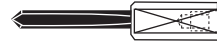
VHW DOWEL DRILLS FOR BOTH RIGHT HAND AND LEFT HAND ROTATION Z=1 Page 5.16
