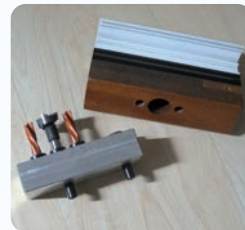
• DRILLING OF WOOD AND PVC • WINDOW FRAME TO • FIT CREMONE BOLT • Page 16.13
