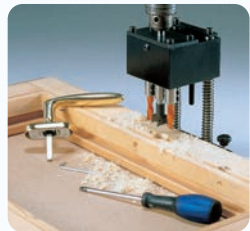
• DRILLING JIG FOR CREMONE BOLTS • Page 16.09
