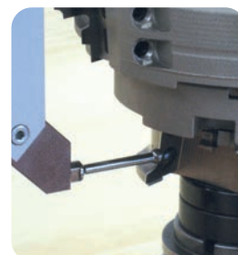
Spherical feeler for shaped cutters (Optional)
